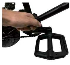
C. Insert R" pedal into right crank arm thread turning clockwise to tighten using 15mm spanner and ensure both pedals are tight.
