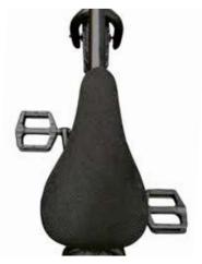
central with top tube of the frame and tighten seat clamp with 6mm hex key.
