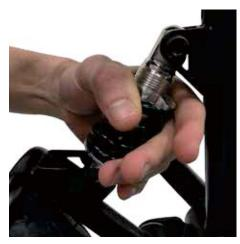
Depending on the weight of the user the spring tension may need to be adjusted by hand, this is all up to the riders preference. (Tightening= harder)(loosening= softer).
