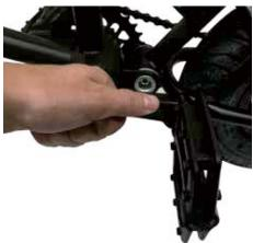
B. Insert L" pedal into left crank arm thread turning anti clockwise to tighten using 15mm spanner.
