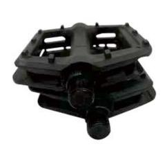
A. Remove pedals from plastic. Indicated on the thread of the pedals says L" or R".
