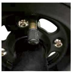
Insert seat into the frame, align seat saddle Remove valve cap located in the inner rim of either wheel, pump wheel up to 30 P.S.I. using appropriate pump for standard bike valve.
