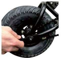
Check the bolts that were pre-tightened/ assembled and ensure they are tight and secure.
