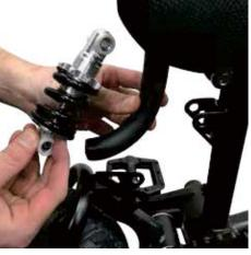
Using 6mm hex key and the 13mm spanner remove nuts and bolts holding the spring attachment, replace spring attachment with solid attachment and reinstall nuts and bolts ensuring they are tight and secure.
