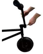
C. Align handle bar approximately with the fork angle and tighten 4 bolts with 6mm hex key till tight and secure.
